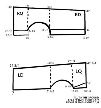
The maximum combined length of door and quarter together, front to back, is as follows:
