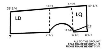
The maximum combined length of door and quarter together, front to back, is as follows:
